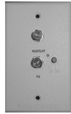
Antenna Power Supply
