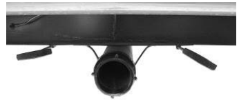
Black/Grey Tank Drain and Valves
